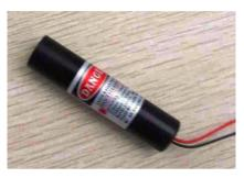
The dimensions of these small laser diode ±modules and YAG- lasers are typically 12 mm diameter and approximately 40 mm in length. Special optics can be used to create contours such as lines, crosses, grid patterns etc. Using an additional galvoscanner any contours can also be created software controlled.
